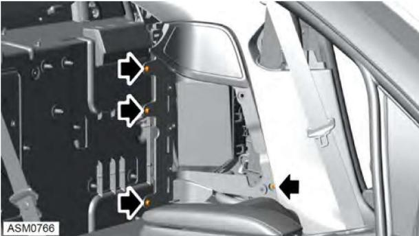
3. Remove M6x20 bolts (x3) securing rear quarter trim to rear bulkhead. **Torque 7 Nm.**
