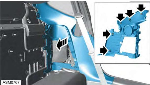
5. Carefully pull rear quarter trim to disengage clips (x5) securing trim panel to bodyside panel.
